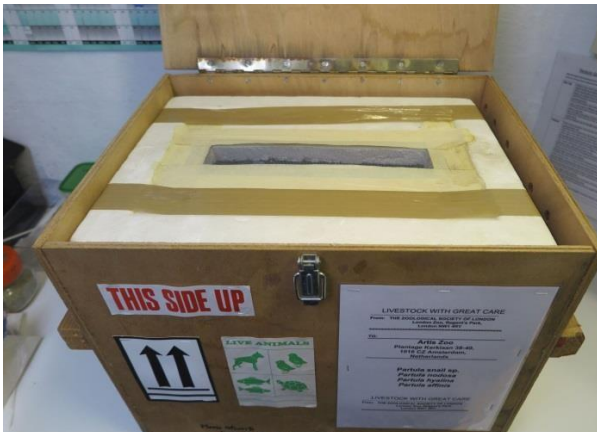
1cm thick plywood crate with 2cm thick inner polystyrene box with ventilated lid
