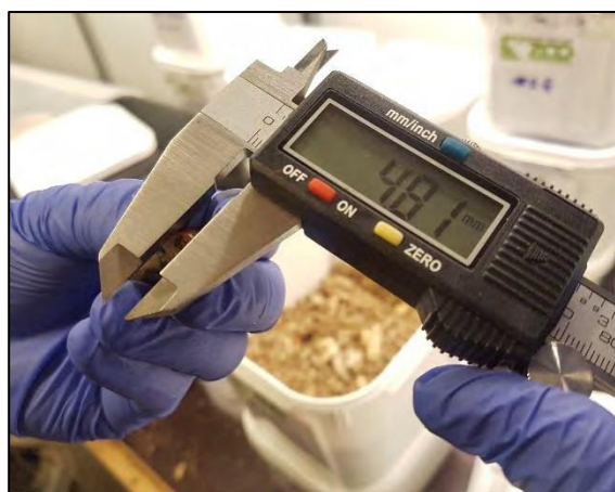
Figure 4. Measurement of HCW of a larva using a digital caliper.
