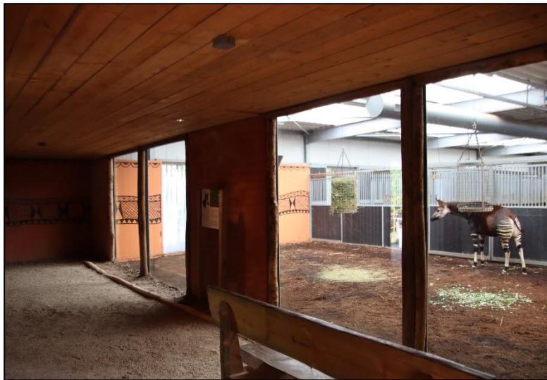
Figure 49 – For indoor facilities, glass is an effective barrier to provide a quiet environment to the animals while still allowing the visitors to see them when kept inside. @João Pedro Meireles / Location: Safaripark Beekse Bergen.
