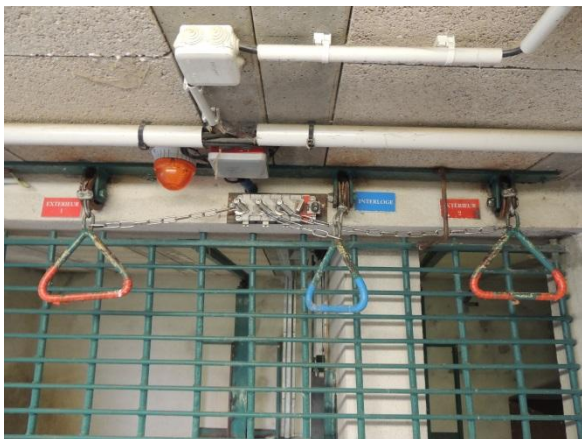
Figure 31: Secure system for the animal access hatches at Obterre zoo © P. Roux
