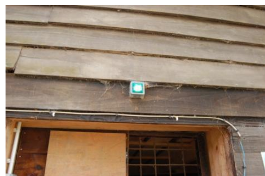
Figure 29: Green light on when all the boxes are well locked up © CERZA zoo
