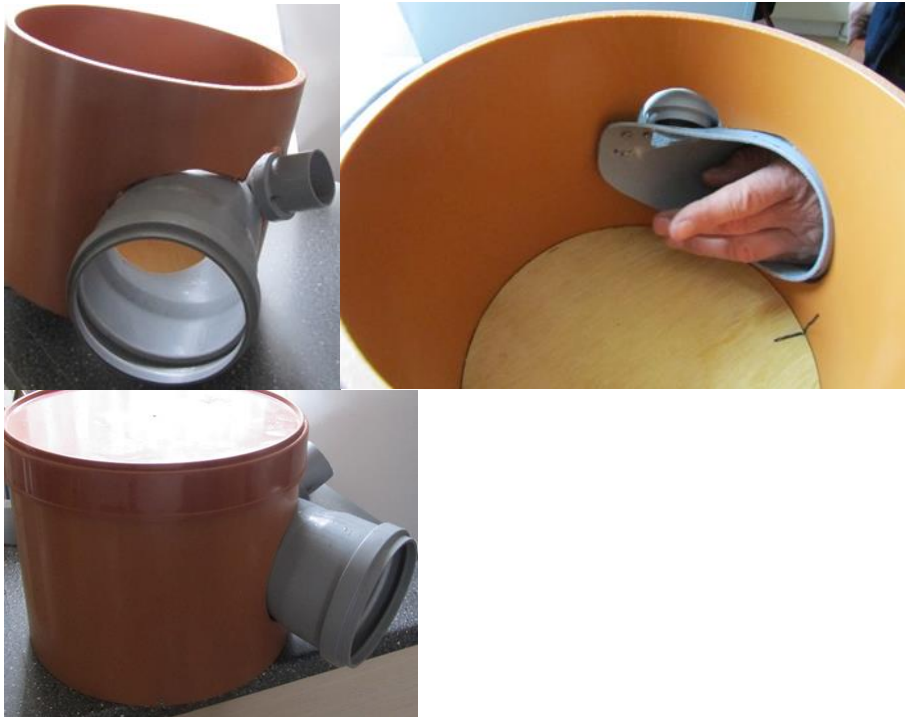
Artificial nest boxes used for fieldwork in breeding colonies of Puffins on the Faroe Islands. Useable for captive breeding too. Right small tube for camera access to the nest. Imbedded in the rock work or ground. Extend entrance onto 80 cm. Nest Ø 30cm, height 35 cm. Entrance Ø 10 – 12 cm. (Photos: F. Nielsen)
