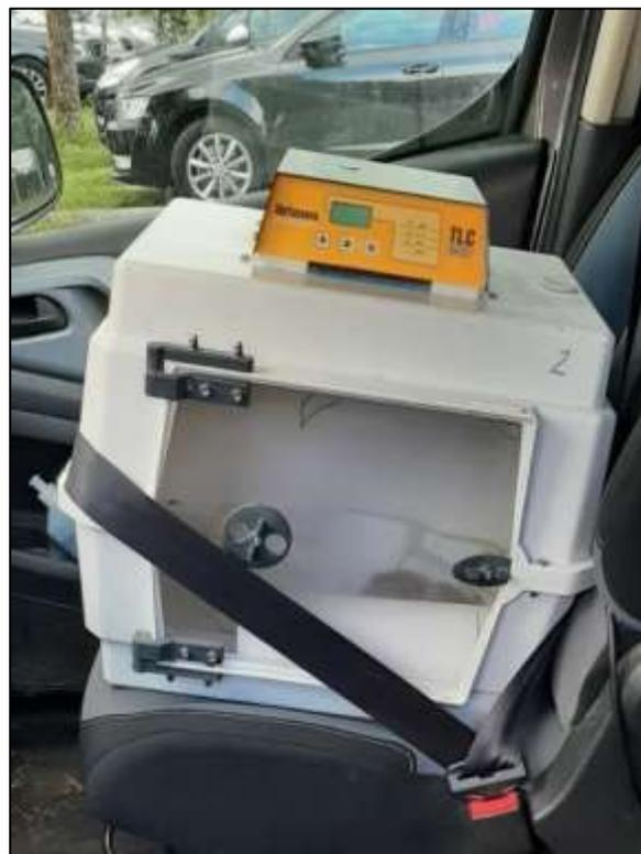
Figure 81 Brinsea Brooder TLC-40 – with transformer for use in the car.
