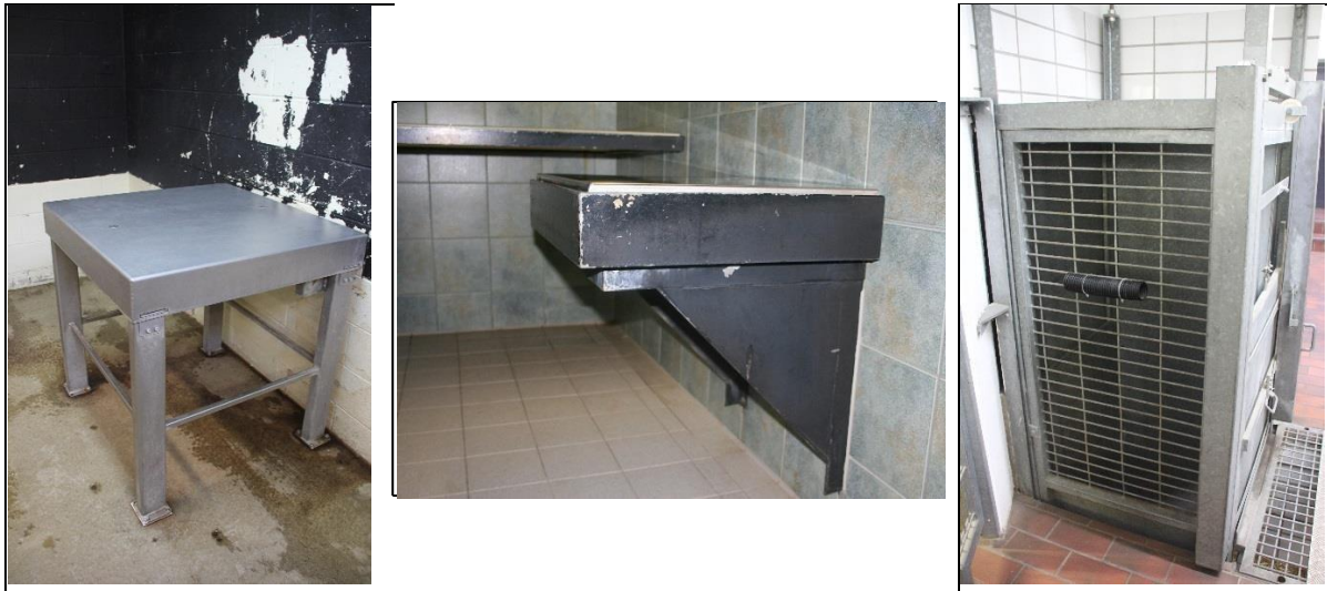
Figure 57: Different models of weighing devices used for bonobos: a: Table model (Columbus Zoo – Jeroen Stevens); b: Integrated in sleeping platform (Leipzig Zoo – Jeroen Stevens); c: A hanging cage in which the bonobos climb and sit (Wuppertal Zoo – Jeroen Stevens).
