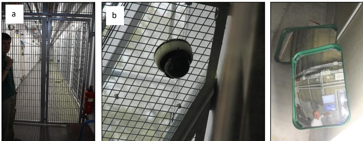
Figure 59: Safety measures to increase visibility or safety in service corridors. a: safety doors (Wilhelma Zoo Stuttgart–Jeroen Stevens); b: safety cameras (Wilhelma Zoo Stuttgart–Jeroen Stevens); c: Safety mirror to avoid blind angles (Wilhelma Zoo Stuttgart–Jeroen Stevens).
