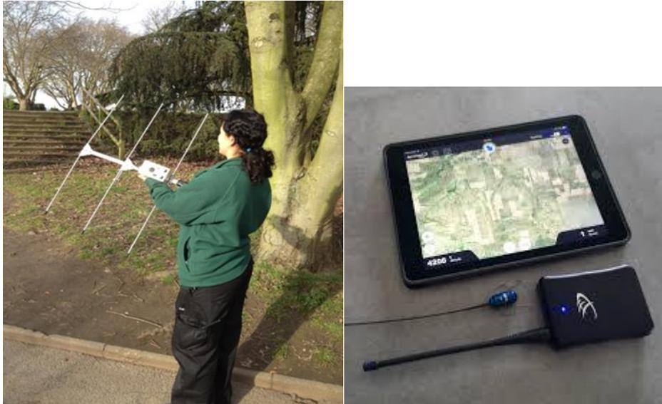
Figures 17 and 18 showing a typical receiver used to locate a transmitter and a new GPS system that links with GPS technology in smart phones and tablets.
