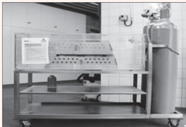
Figure 3 Plastic container, designed to hold several typical rodent transport boxes, linked to CO<sub>2</sub> gas bottles.
